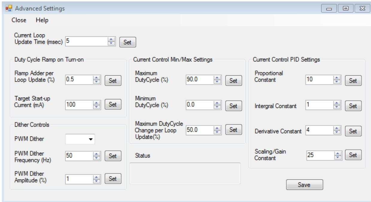
Model 805 – Configuration and Control User Interface, Advanced Parameter Screen
